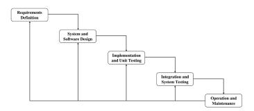
Figure 1. Waterfall Method System Development Life Cycle (SDLC) Flow
