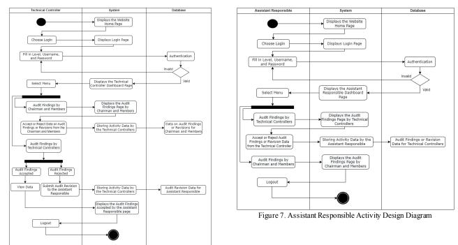
Figure 6. Technical Controller Activity Design Diagram
