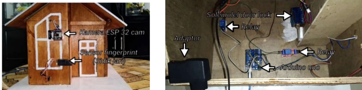
Figure 2. Smart Door Lock Prototype
