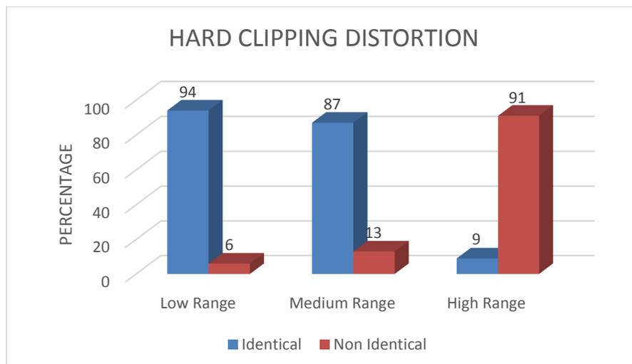
Figure 11. Percentage of results from hard clipping distortion
